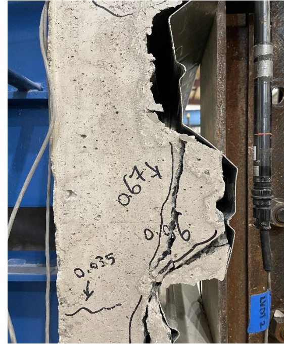
Rib Shear/Concrete Cone
