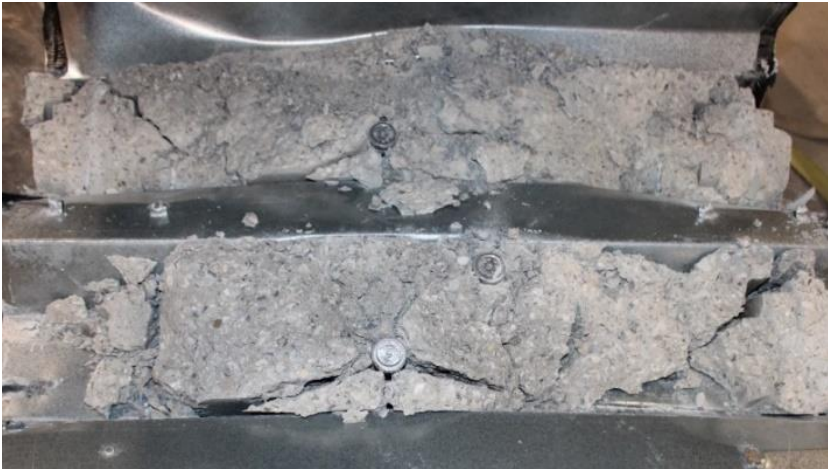
Plan View of Concrete Cone After Testing
