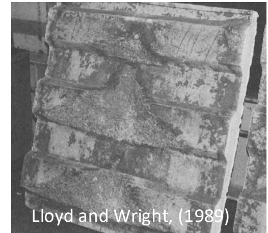
2. Concrete Pullout Failure
