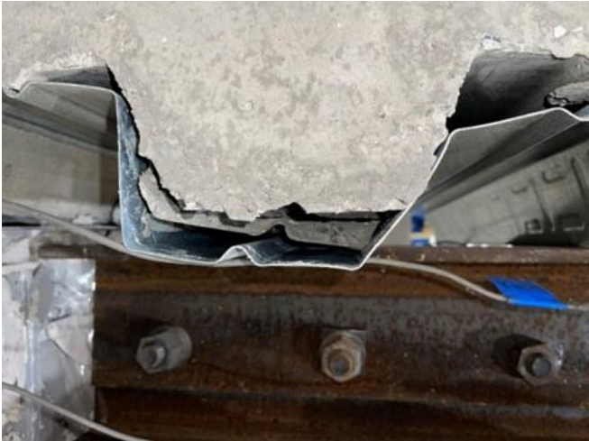
Plan View of Concrete Cone After Testing
