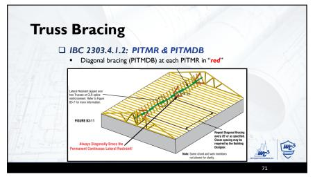
**Truss Bracing** ☐ IBC 2303.4.1.2: PITMR & PITMDB When the truss plans call for PITMR, it must be provided by one of following... 1. PITMR & PITMDB shall be provided using standard industry lateral restraint and diagonal bracing details per TPI, accepted engineering practice, or Figures 2303.4.1.2(1), (3), and (5). 2. Buckling reinforcement is added to individual truss per truss drawings, or per Figures 2303.4.1.2 (2) and (4). 3. Project-specific PITMR and PITMDB design by EOR. **ADDED**
